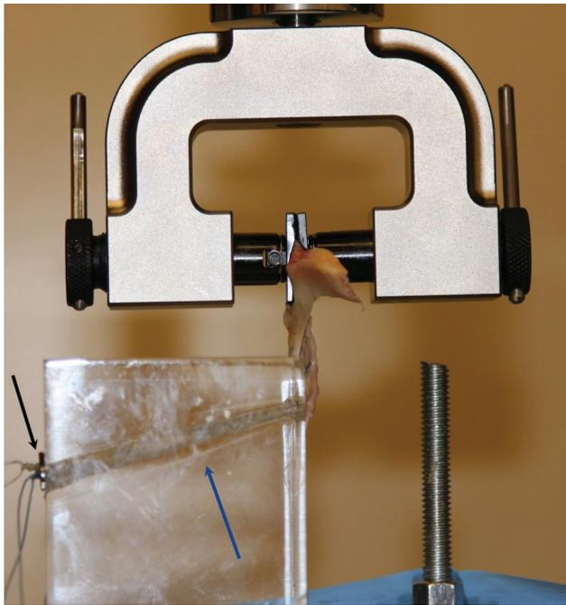
**Figure 3.** Uniaxial testing construct. The left arrow points to the suture button, and the right arrow points to the tunnel through an acrylic jig.
