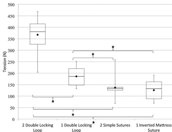
**Figure 5.** Box plot of the maximum failure load of 4 meniscal repair constructs. Brackets with stars represent statistically significant interconstruct comparison. The y-axis represents tension (in newtons).
